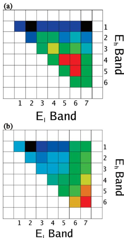
**Figure 7.** Frequency plot for interband transitions (i.e., between the band of minima containing the higher-energy minimum ( $E_h$ ) and the band containing the lower-energy minimum ( $E_l$ )) for  $M_{13}$  clusters,  $\rho = 5$ : (a) absolute frequencies, color ranging from 27 (black) to 846 (red); (b) normalized frequencies, color ranging from  $-2.56$  (black) to 1.40 (red).
