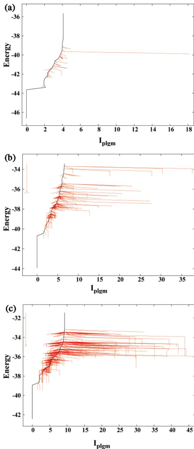
**Figure 3.** Disconnectivity graphs using the average integrated path length of minima from the GM ( $I_{\text{plgm}}$ ) within basins to position the basins on the  $x$ -axis, using an energy increment of 0.25: (a)  $\rho = 4$ ; (b)  $\rho = 5$ , and (c)  $\rho = 6$ . The basin containing the global minimum is shown in black, whereas all other basins are shown in red.
