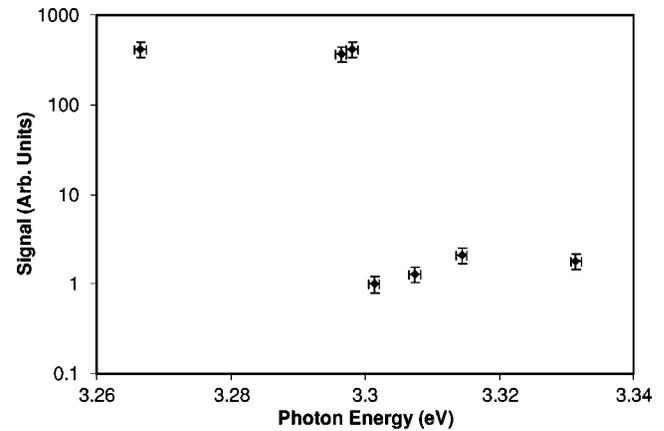
FIG. 6. The energy dependence of three-photon absorption for atomic Mg as a function of photon energy. The  $3s$  threshold lies at 3.3004 eV above the  $3\ ^1P$  state.
