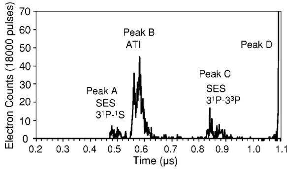
FIG. 2. A two-color time-of-flight spectrum. Peak A is caused by SES of electrons from  $3\ ^1P$  Mg to  $3\ ^1S$ , peak B is caused by two-photon ATI from the  $3\ ^1P$  state, peak C is caused by SES from  $3\ ^1P$  to the  $3\ ^3P$  state, and peak D is REMPL.
