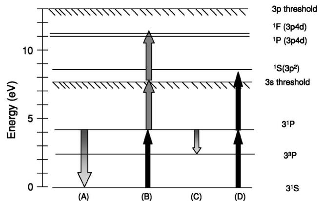
FIG. 1. A sketch of the relevant energy levels and processes studied in this paper. The dark arrows indicate the 285.21-nm light, the gray arrows indicate the nonresonant photons, and the shaded arrows indicate the deexcitation due to superelastic scattering.
