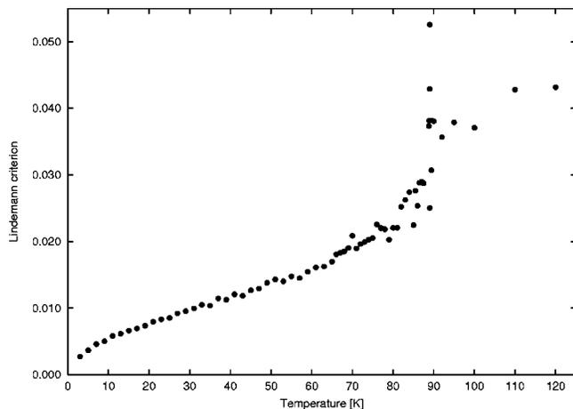
FIG. 6. Lindemann index for  $(\text{TeF}_6)_{89}$  clusters: The slope of the curve changes in the region of 60 K indicating a continuous transition. The jump at  $\approx 90$  K shows lattice reconstruction but the cluster is solid.
