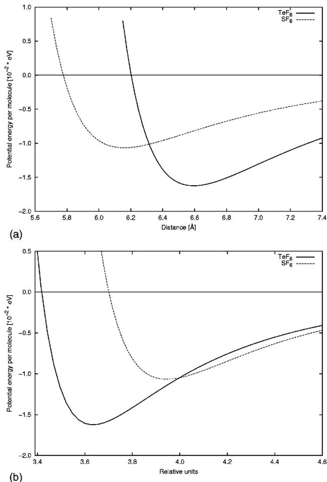
FIG. 1. Pairwise potentials for TeF<sub>6</sub> and SF<sub>6</sub> molecules.
