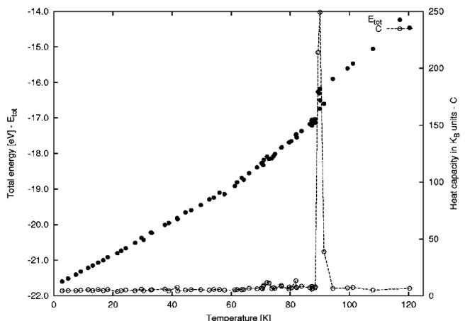
FIG. 3. Caloric curve and the heat capacity for a  $(\text{TeF}_6)_{89}$  cluster. The heat capacity is computed from the energy fluctuations and is plotted in  $k_B$  units.
