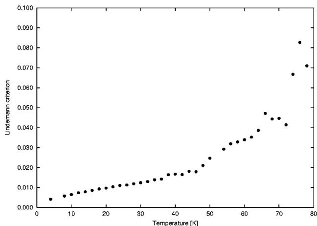
FIG. 5. Lindemann index for  $(\text{SF}_6)_{89}$  clusters: Solid–solid transformations are observed at  $\approx 40$  K and  $\approx 60$  K. The jump at  $\approx 80$  K shows the solid–liquid transition.
