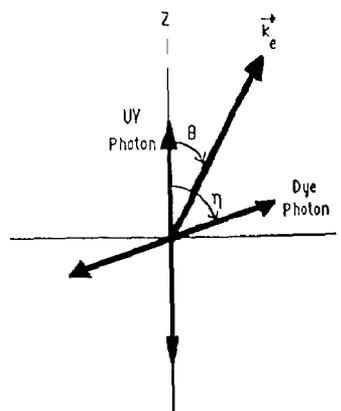
Fig. 2. Schematic of the system geometry. The collinear plane-polarized laser beams, propagating out of the page, intersect the molecular beam at the origin. The polarization vector of the ionizing beam defines the  $z$  axis; the angle between the polarization vectors of the ionizing and exciting laser beams is denoted  $\eta$ . The momentum vector  $k_e$  of the photoelectron is in the plane of the paper at an angle  $\theta$  from the  $z$  axis.
